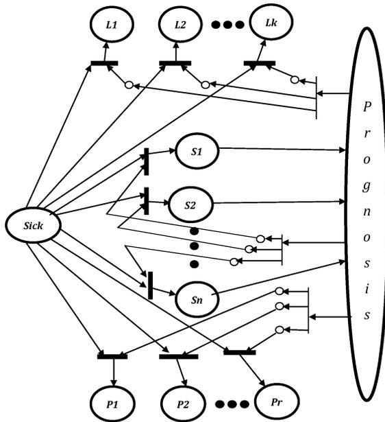
Fig. 8. SPN state diagram of the user's health conditions. The circles represent states, the thick lines represent transitions (associated with probabilities), and the arrows represent the flow of the tokens that reflect the operation of the model and the transitions from one state to other states.
