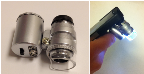
Figure 3. a) Microscope with 60x zoom capability designed for the iPhone 4/4S. b) Microscope mounted on the iPhone while in use (LED light is on)
