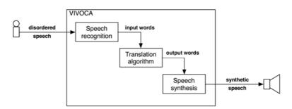
Figure 1. System diagram of the voice-input voice-output communication aid (VIVOCA).
