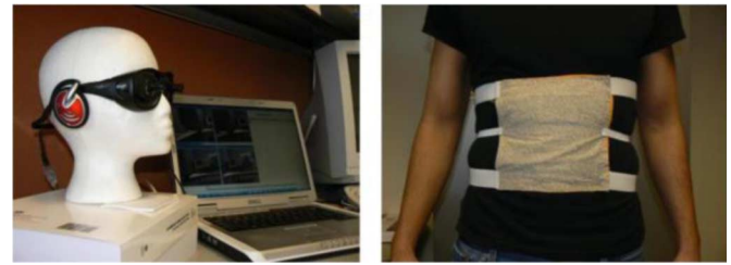
Fig. 17. Tyflos' second prototype hardware components. Left: stereo cameras attached on dark eyeglasses, microphone, earphones, and portable computer. Right: 2-D vibration array vest attached on a user's abdomen.
