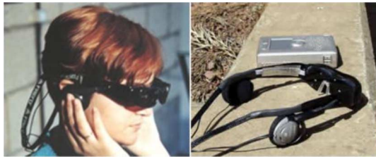
Fig. 6. Virtual acoustic space prototype (cameras and headphones mounted on eyeglasses and microprocessor) (right).
