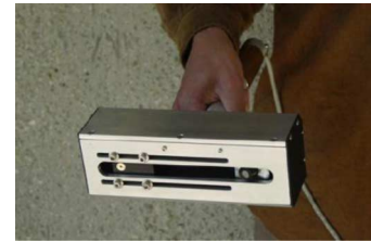
Fig. 19. UCSC's handheld device equipped with laser range sensor.
