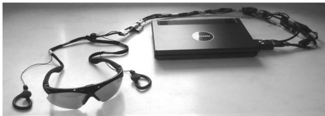
Fig. 3. Implementation of the vOICE—“Seeing with sound” system (glasses with attached camera, earspeakers, and portable computer).
