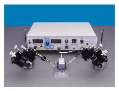
Figure 2: Voltage Clamp Apparatus Two Electrode Voltage Clamp Apparatus. From https://www.warneronline.com/product\_info.cfm?name=TEV-700+Two+Electrode +Voltage+Clamp+Workstation&id=170.
